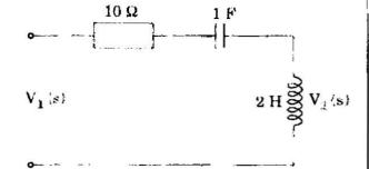
The driving point impedance of the network shown in figure is
