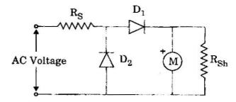
The figure shows the circuit of a rectifier type voltmeter. The diode  $\mathrm{D}_2$
