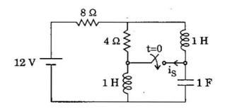
The circuit shown in the figure is in steady state before the switch is closed at t=0. The current  $i_{\rm S}(0^+)$  through the switch is
