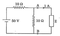
Consider the circuit shown above. The portion of the circuit left to the terminals AB can be replaced by
