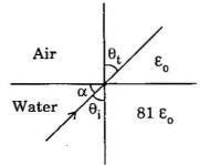
A plane wave is generated under water  $(\epsilon=81~\epsilon_0$  and  $\mu=\mu_0)$ . The wave is parallel polarized. At the interface between water and air, the angle  $\alpha$  for which there is no reflection is
