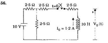
In the circuit shown, the initial current  $l_0$  through the inductor is given in the figure. The initial value of the voltage across the inductor  $V_0(0^+)$  is
