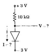
For the circuit shown above, using ideal diode, the values of voltage and current are
