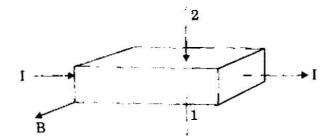
Consider a semiconductor carrying current and placed in a transverse magnetic field B, as shown above. The measured potential across 1 and 2 surfaces is positive at 2. What is the type of material?
