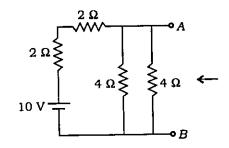
The output resistance of the circuit at port AB is
