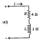
Consider an L-R circuit in which a current  $i = 5e^{-2t}A$  is flowing. The voltage across the R-L circuit is given by
