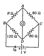
In the circuit shown, when the current through the branch AD is zero, the battery current  $I_B$  is
