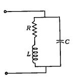
The circuit given above is constituted by an iron-cored coil and a capacitor. At resonance, the circuit behaves like
