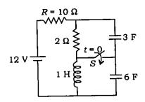
The circuit given above is in steady state for a long time with switch S open. The switch is closed at t = 0. The current through R at t = 0 will be
