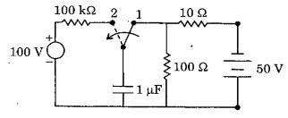
In the above circuit, the switch has been in position 1 for quite a long time. At t=0 the switch is moved to position 2. At this position what is the time constant?
