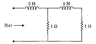
Consider the above network. Impedance of this network as a function of the complex frequency s consists of a certain number of zeros and poles. What is the location of poles?
